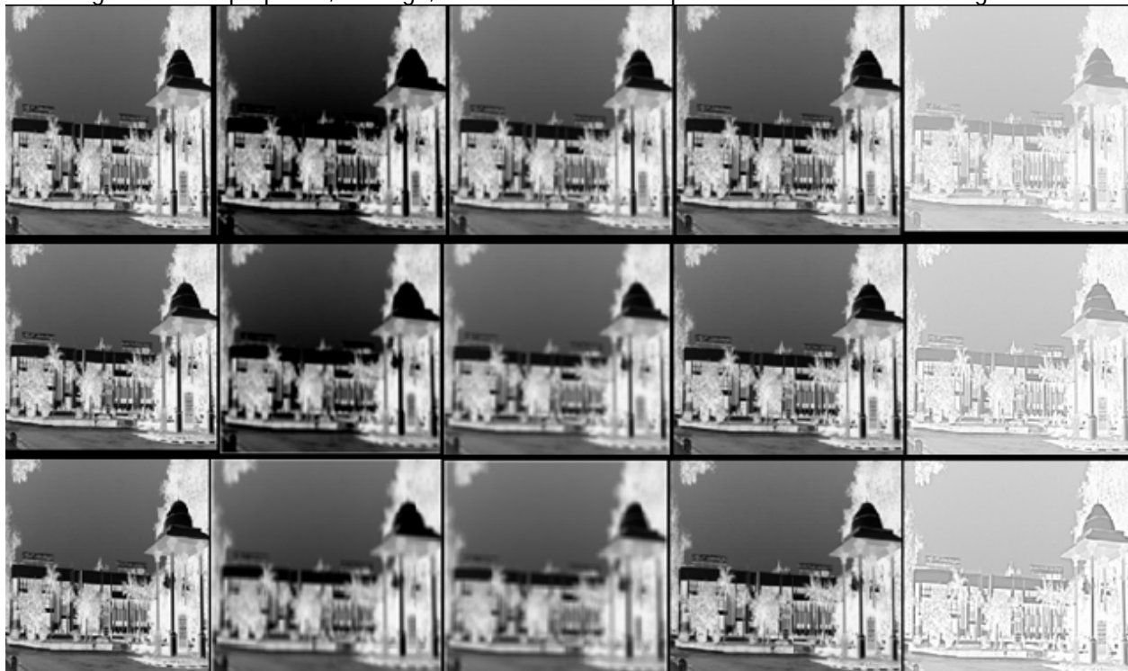
Figure 4. Image results of (a) Original image (b) proposed, (c) average, (d) Gaussian and (e) unsharp filters using 3 \times 3 , 5 \times 5 and 7 \times 7 dimensions
