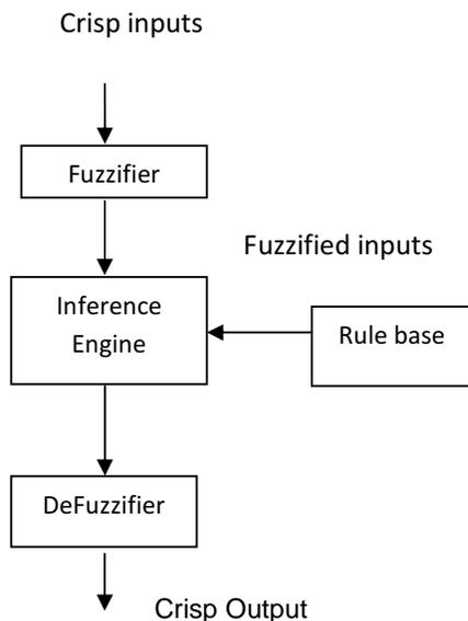
Fig.1. Schematic representation of a Fuzzy System
