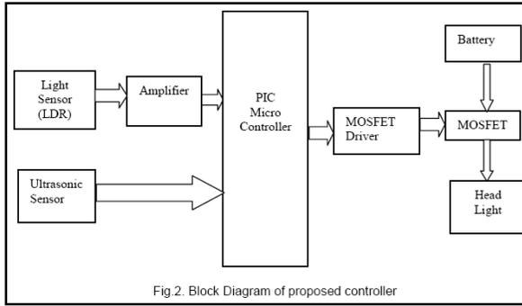
Fig.2. Block Diagram of proposed controller
