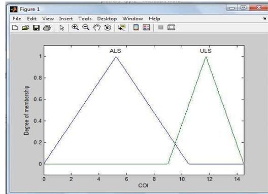
Fig. 12. The membership function for the ControllerOutputIntensity(COI)
