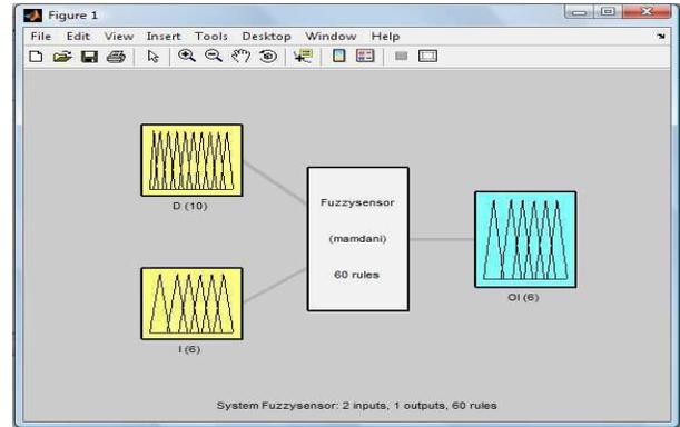
Fig. 4. The structure of the fuzzy sensor
