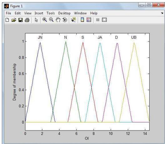
Fig. 7. The membership function of OI(Output Intensity of sensor )
