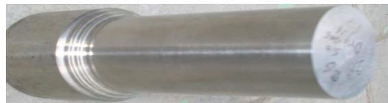
Fig.3: Work-piece Titanium-Ti-6Al-4V
