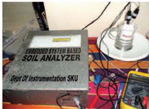
Fig.1. Measurement Of Potassium using Embedded system based Soil Analyzer
