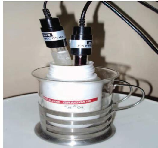
FIG 3: Potassium Sensor electrode and reference electrode are immersed in  $10^{-3}$  M buffer solution
